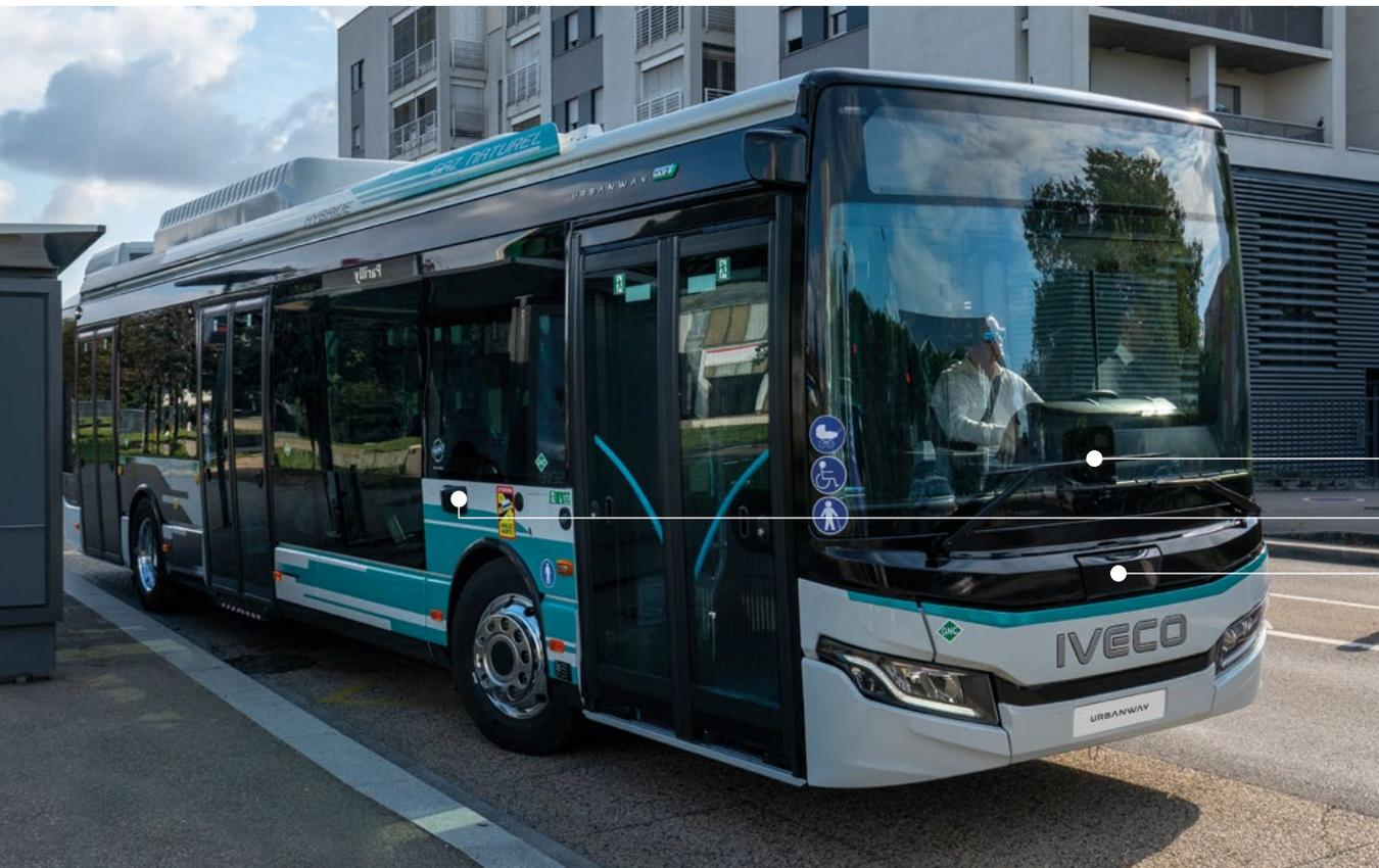
Those sensing tools are incorporated in a radar installed in the front face and a camera lens covering the whole frontal area from the inner side behind the windscreen. Its combination is able to detect Vulnerable Road Users approaching frontally and from lateral directions, as well as road signals. The camera is packed with a light sensor allowing the automatic switching on of front headlights.
