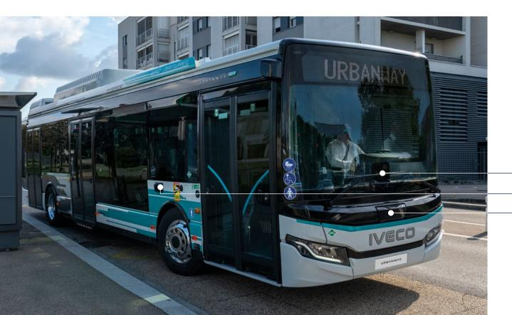
Those sensing tools are incorporated in a radar installed in the front face and a camera lens covering the whole frontal area from the inner side behind the windscreen. Its combination is able to detect Vulnerable Road Users approaching frontally and from lateral directions, as well as road signals.
